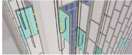
Figure 9. Representation of cleaning chambers with hoses connected roof tanks.
